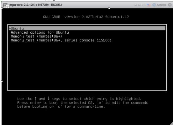
**3.** Using the keyboard Up and Down arrow keys, select **Advanced options for Ubuntu** from the menu and press Enter.
