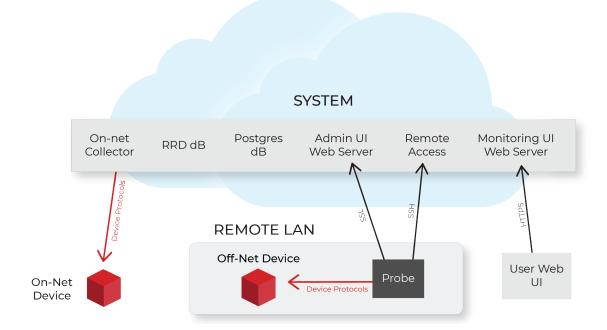
The various Mitel Performance Analytics components can run on a single or multiple servers, depending on capacity requirements.
